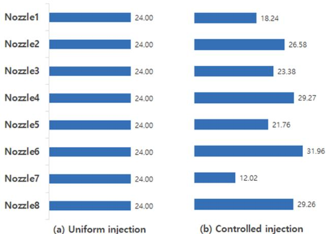
Figure 11. AIG nozzle flow rate for case 1.
